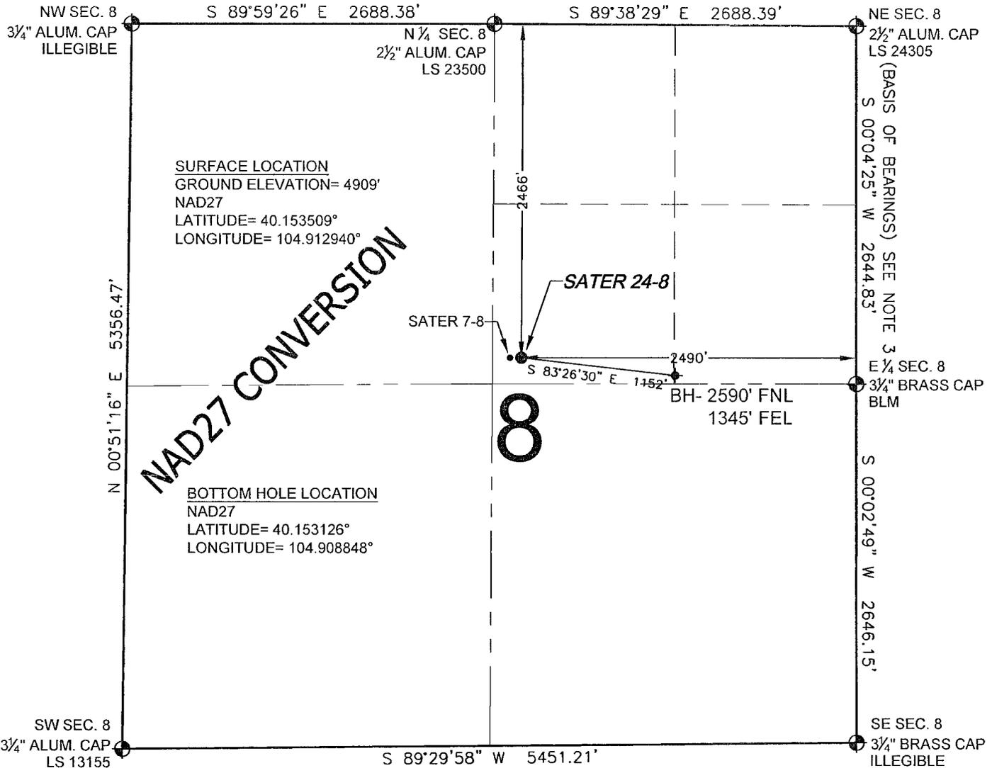
WELL **SATER 24-8** TO BE LOCATED 2466' FNL AND 2490' FEL, SECTION 8, T2N, R67W OF THE 6th P.M.
