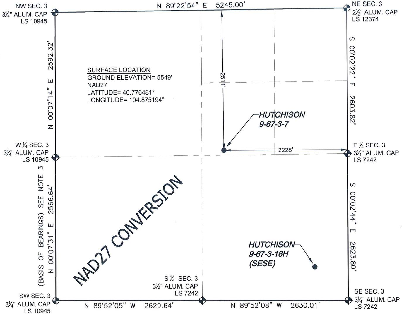
WELL HUTCHISON 9-67-3-7 TO BE LOCATED 2511' FNL AND 2228' FEL, SECTION 3, T9N, R67W OF THE 6th P.M.
