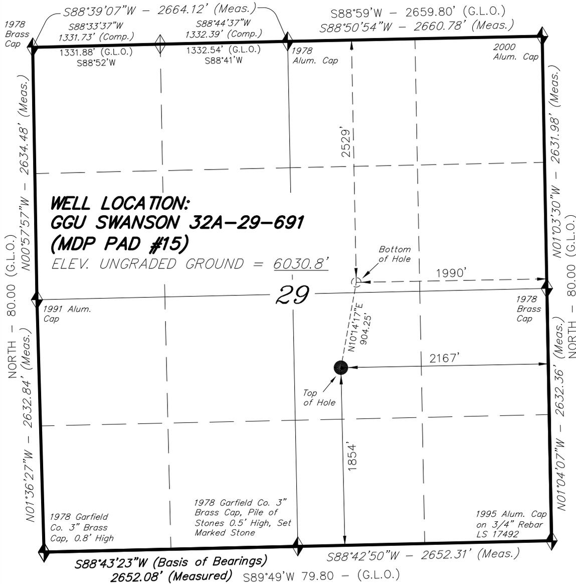
WELL LOCATION, GGU SWANSON 32A-29-691 (MDP PAD #15), LOCATED AS SHOWN IN THE NW 1/4 SE 1/4 OF SECTION 29, T6S, R91W, 6th P.M. GARFIELD COUNTY, COLORADO.
