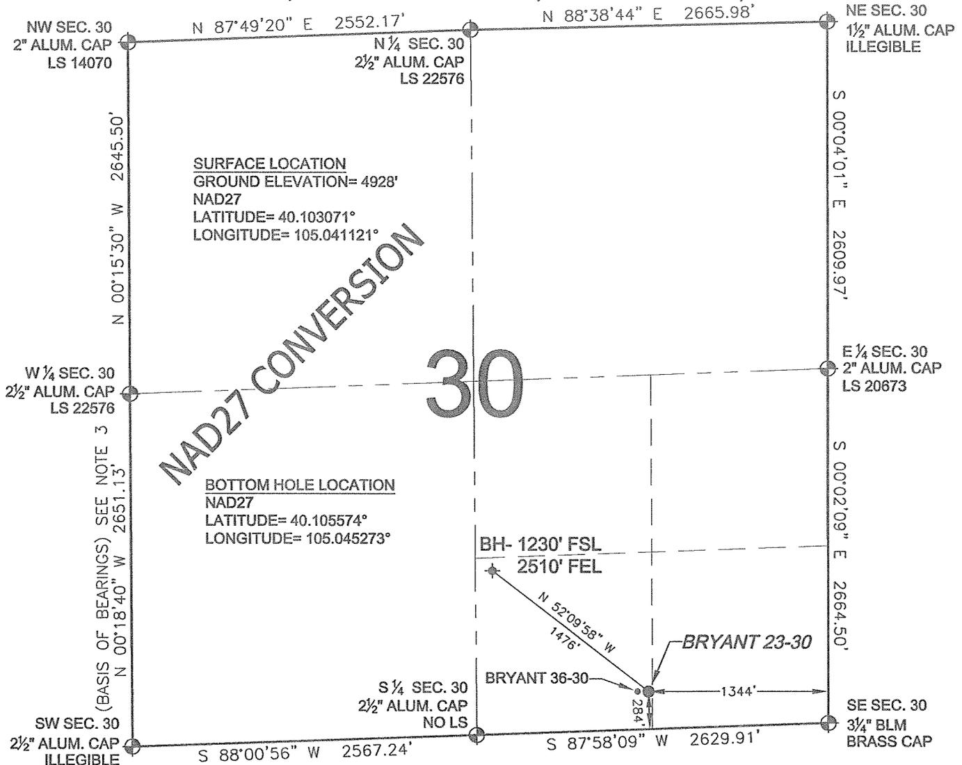
WELL BRYANT 23-30 TO BE LOCATED 284' FSL AND 1344' FEL, SECTION 30, T2N, R68W OF THE 6th P.M.
