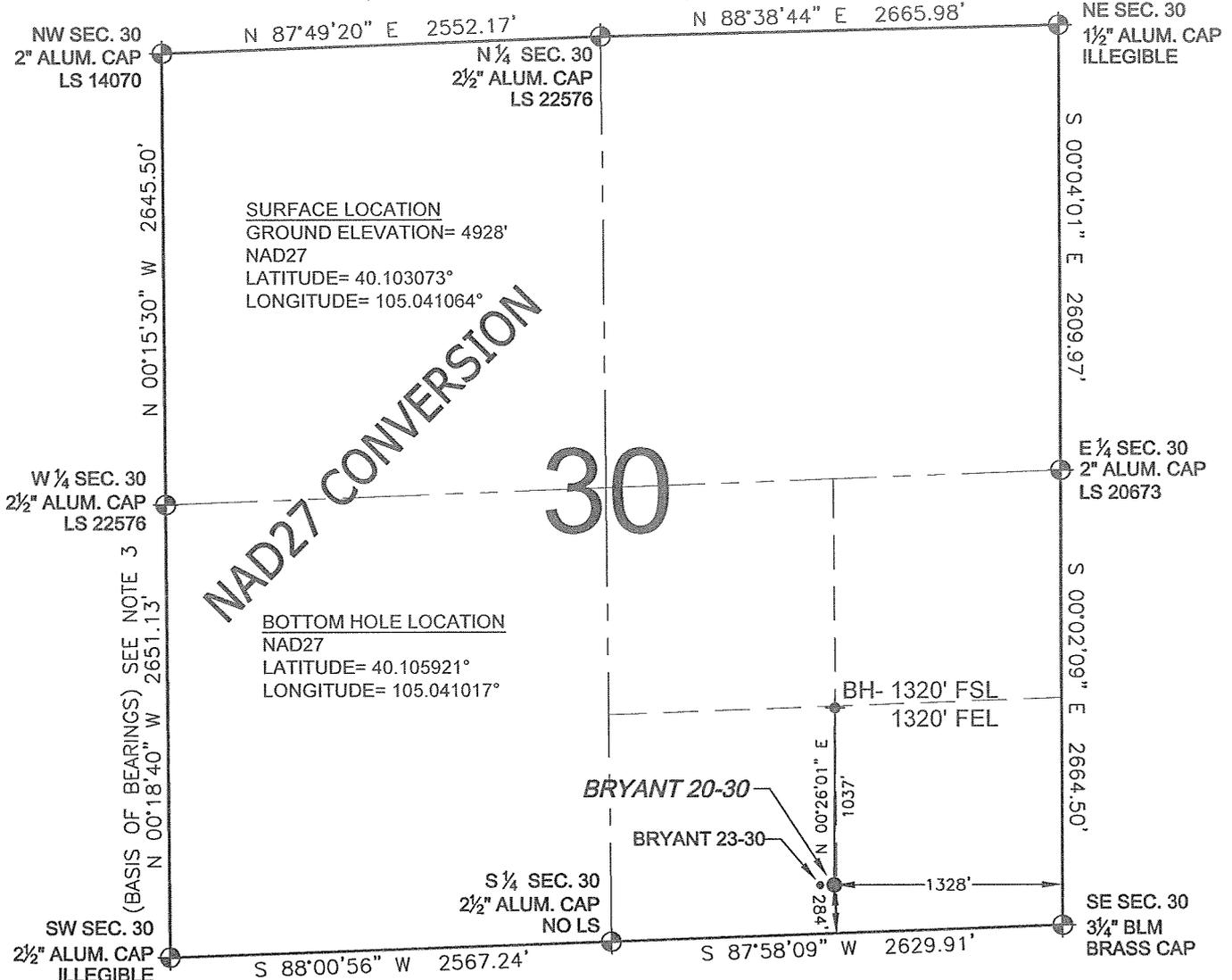
WELL BRYANT 20-30 TO BE LOCATED 284' FSL AND 1328' FEL, SECTION 30, T2N, R68W OF THE 6th P.M.
