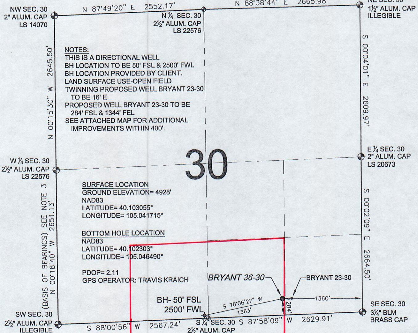
WELL **BRYANT 36-30** TO BE LOCATED 284' FSL AND 1360' FEL, SECTION 30, T2N, R68W OF THE 6th P.M.
