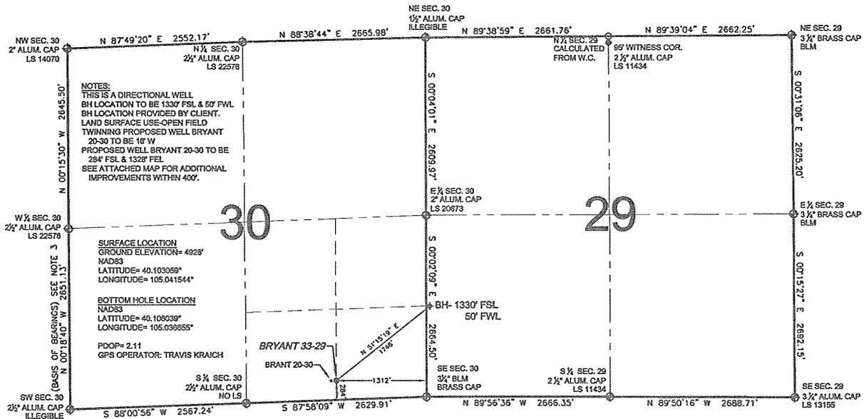
WELL BRYANT 33-29 TO BE LOCATED 284' FSL AND 1312' FEL, SECTION 30, T2N, R68W OF THE 6th P.M.
