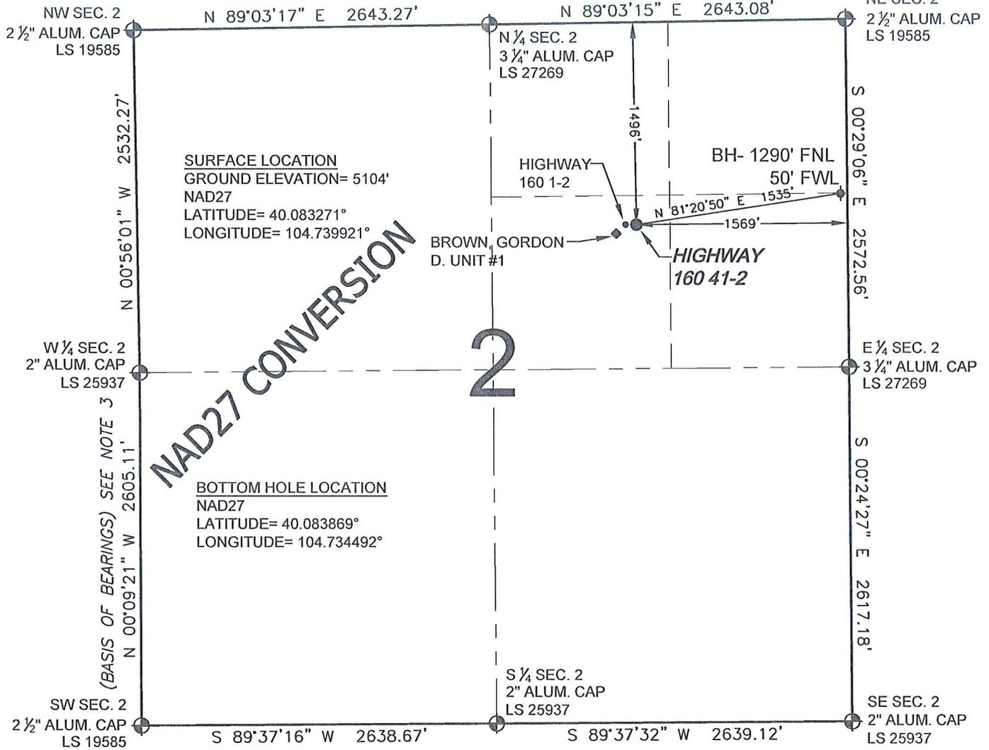
WELL HIGHWAY 160 41-2 TO BE LOCATED 1496' FNL AND 1569' FEL, SECTION 2, T1N, R66W OF THE 6th P.M.
