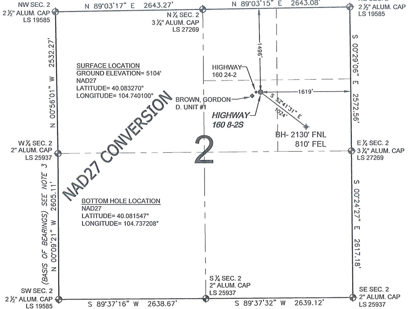
WELL HIGHWAY 160 8-2S TO BE LOCATED 1496' FNL AND 1619' FEL, SECTION 2, T1N, R66W OF THE 6th P.M.
