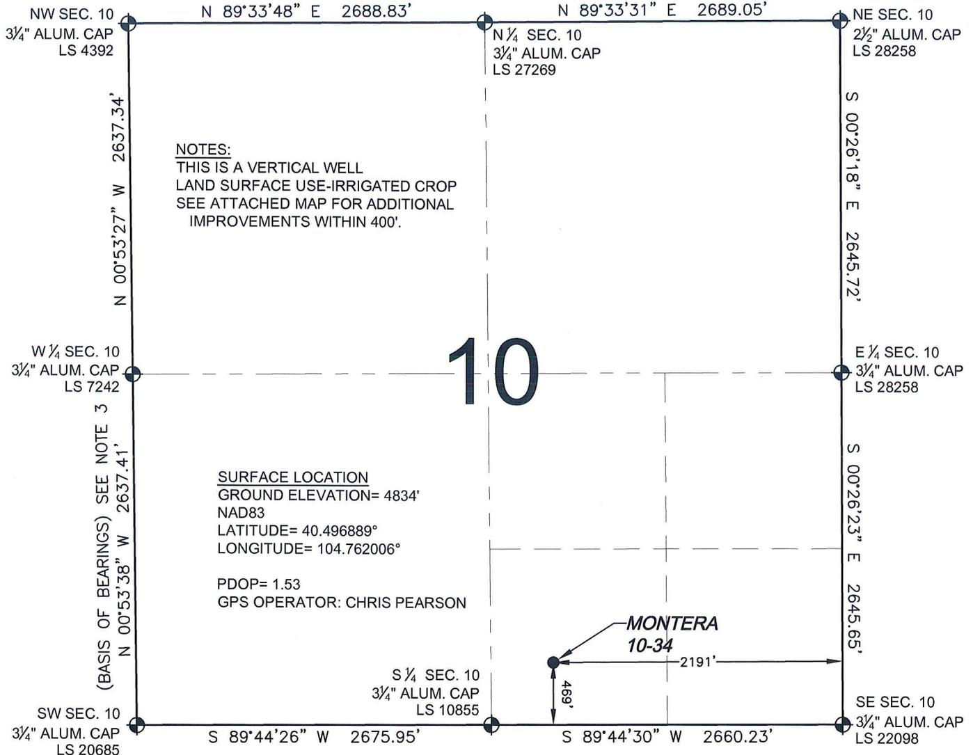
WELL **MONTERA 10-34** TO BE LOCATED 469' FSL AND 2191' FEL, SECTION 10, T6N, R66W OF THE 6th P.M.
