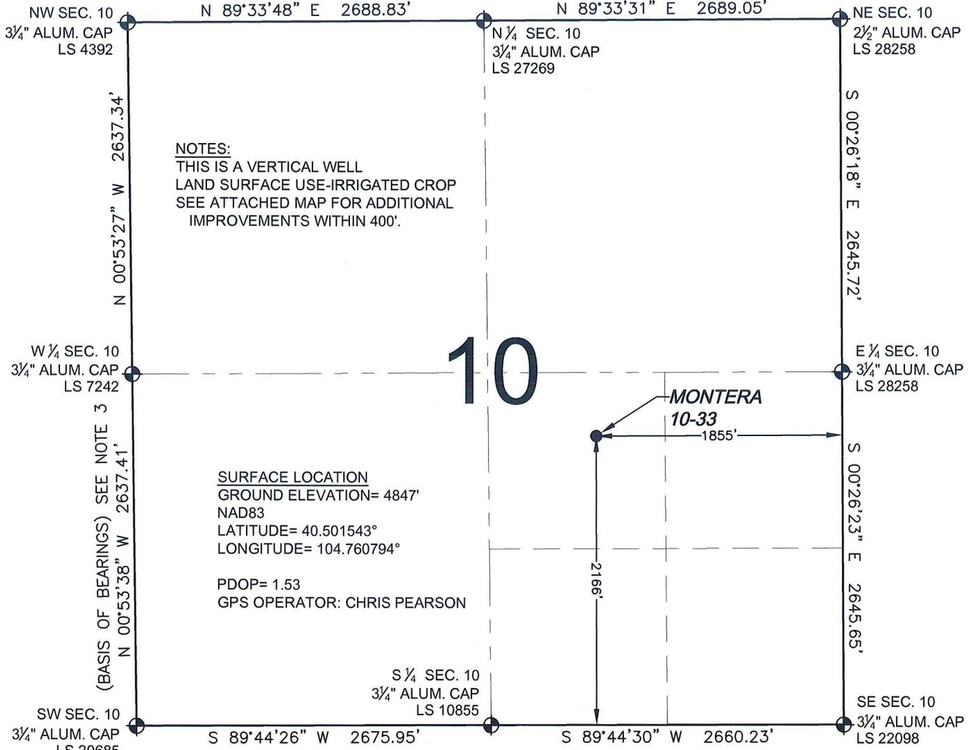
WELL **MONTERA 10-33** TO BE LOCATED 2166' FSL AND 1855' FEL, SECTION 10, T6N, R66W OF THE 6th P.M.
