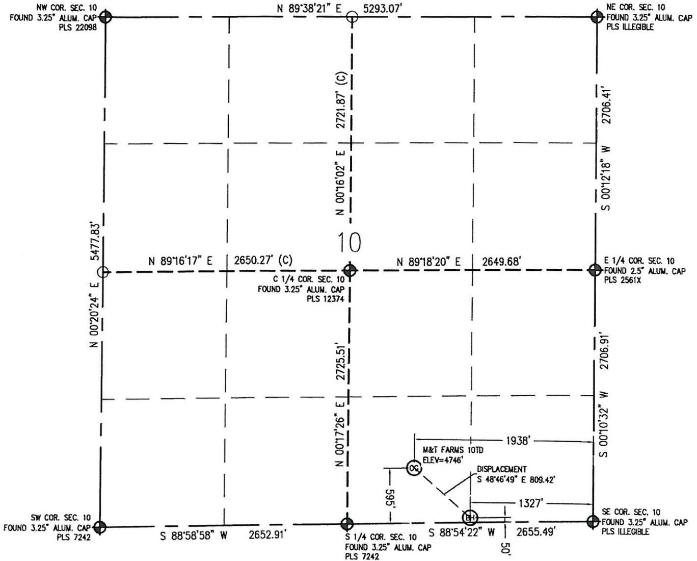
IN ACCORDANCE WITH A REQUEST FROM CRAIG RASMUSON - SYNERGY RESOURCES, BASELINE ENGINEERING CORP. HAS DETERMINED THE LOCATION OF THE M&T FARMS 10TD TO BE 595' FSL AND 1938' FEL, AS MEASURED AT NINETY (90) DEGREES FROM THE SECTION LINE OF SECTION 10, TOWNSHIP 6 NORTH, RANGE 65 WEST AND THE BOTTOM HOLE LOCATION TO BE 50' FSL AND 1327' FEL OF SECTION 10, TOWNSHIP 6 NORTH, RANGE 65 WEST, 6TH PRINCIPAL MERIDIAN, WELD COUNTY, COLORADO.
