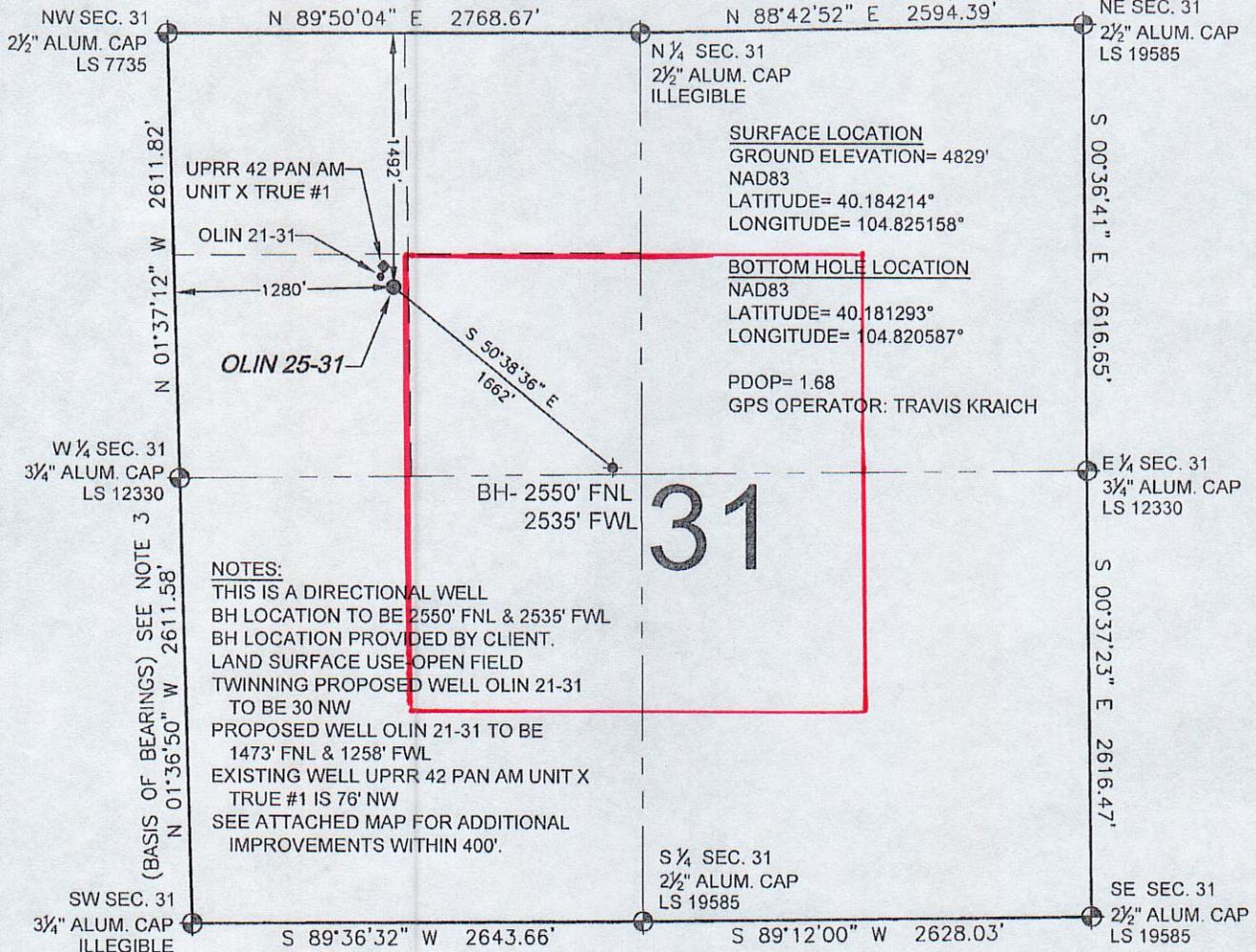
WELL OLIN 25-31 TO BE LOCATED 1492' FNL AND 1280' FWL, SECTION 31, T3N, R66W OF THE 6th P.M.
