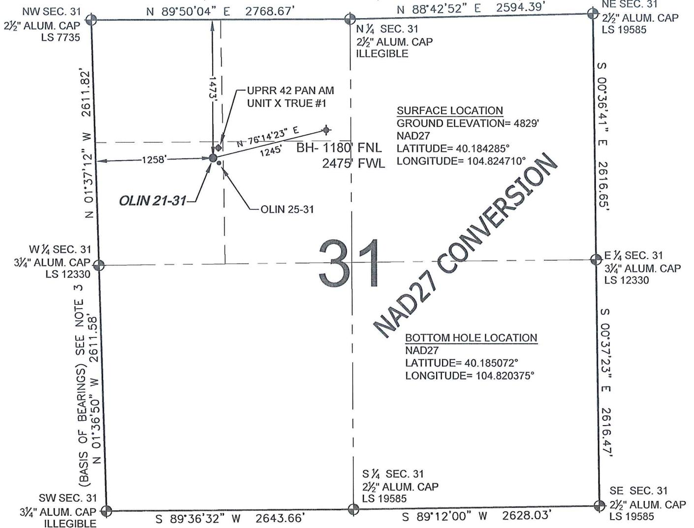
WELL **OLIN 21-31** TO BE LOCATED 1473' FNL AND 1258' FWL, SECTION 31, T3N, R66W OF THE 6th P.M.
