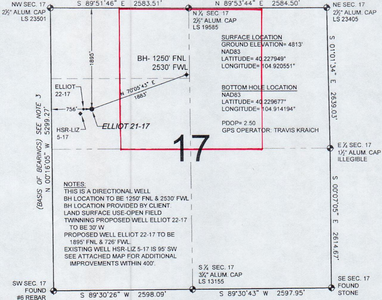
WELL ELLIOT 21-17 TO BE LOCATED 1895' FNL AND 756' FWL, SECTION 17, T3N, R67W OF THE 6th P.M.
