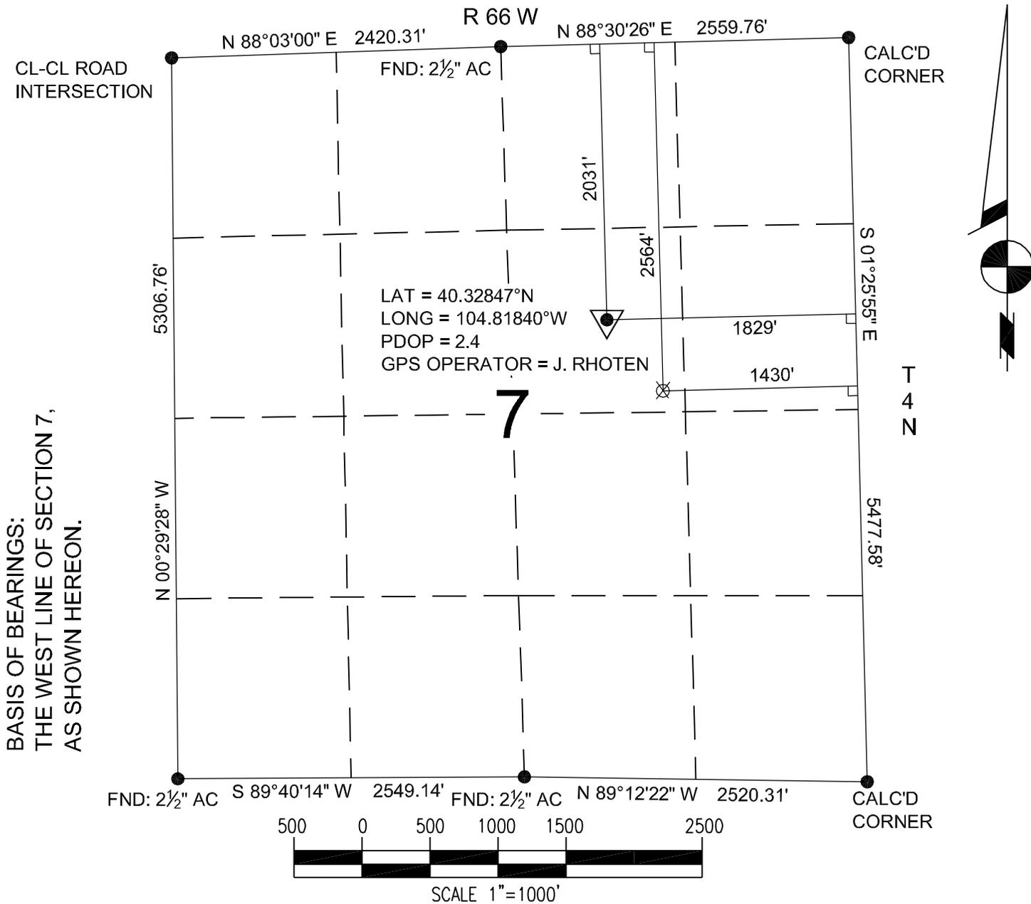
Power Surveying Co., Inc. of Frederick, Colorado has in accordance with a request from SHERRY GLASS for KP KAUFFMAN determined the location of KAMMERZELL 7-7-24 to be 2031' FNL & 1829' FEL Section 7, Township 4 NORTH Range 66 WEST of the Sixth Principal Meridian, WELD County, Colorado
