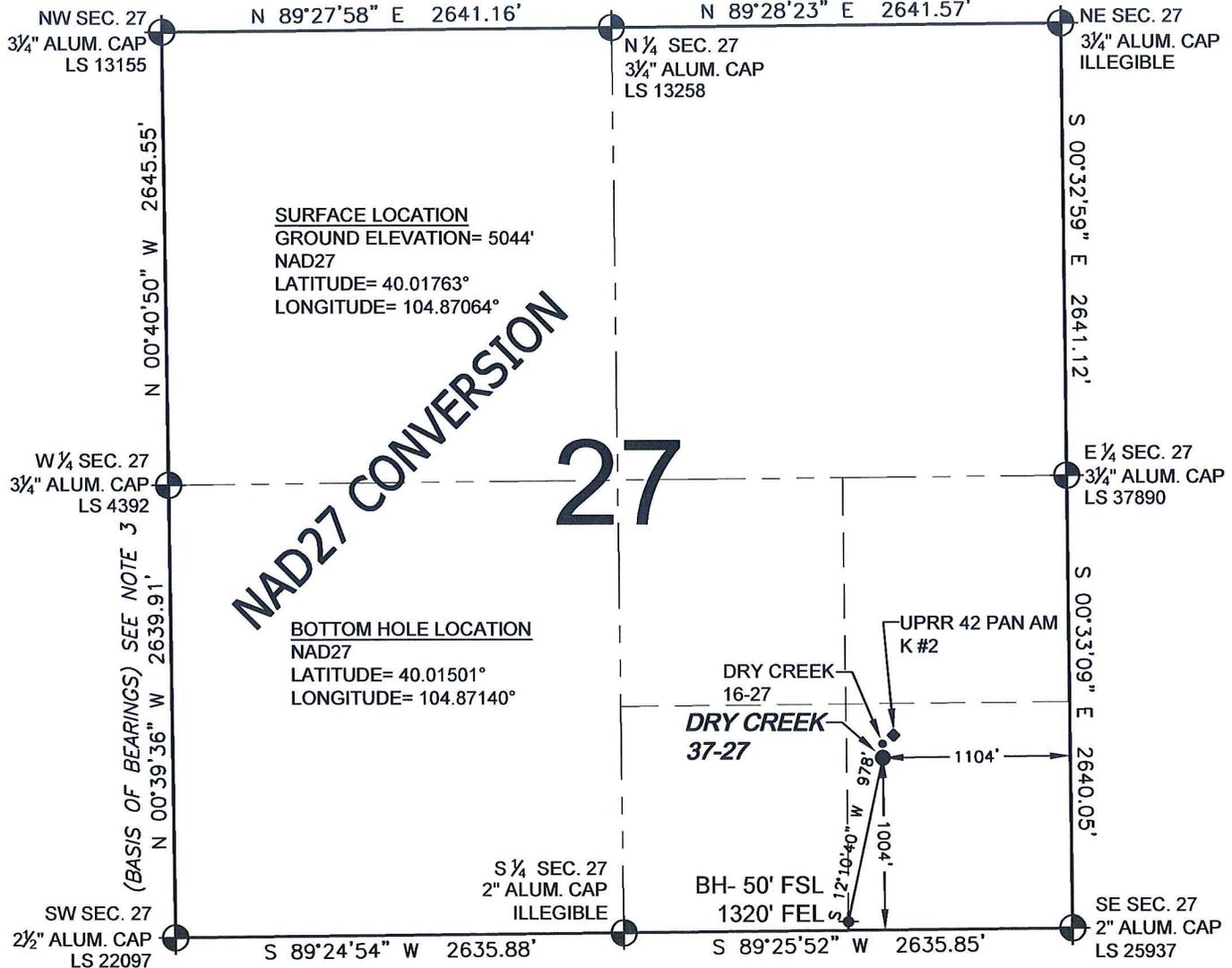
WELL DRY CREEK 37-27 TO BE LOCATED 1004' FSL AND 1104' FEL, SECTION 27, T1N, R67W OF THE 6th P.M.
