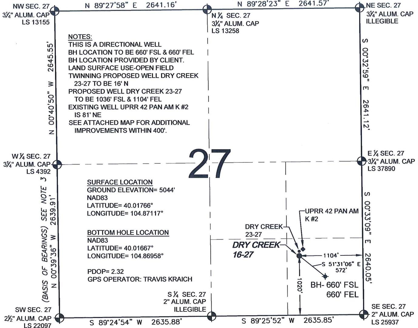
WELL DRY CREEK 16-27 TO BE LOCATED 1020' FSL AND 1104' FEL, SECTION 27, T1N, R67W OF THE 6th P.M.
