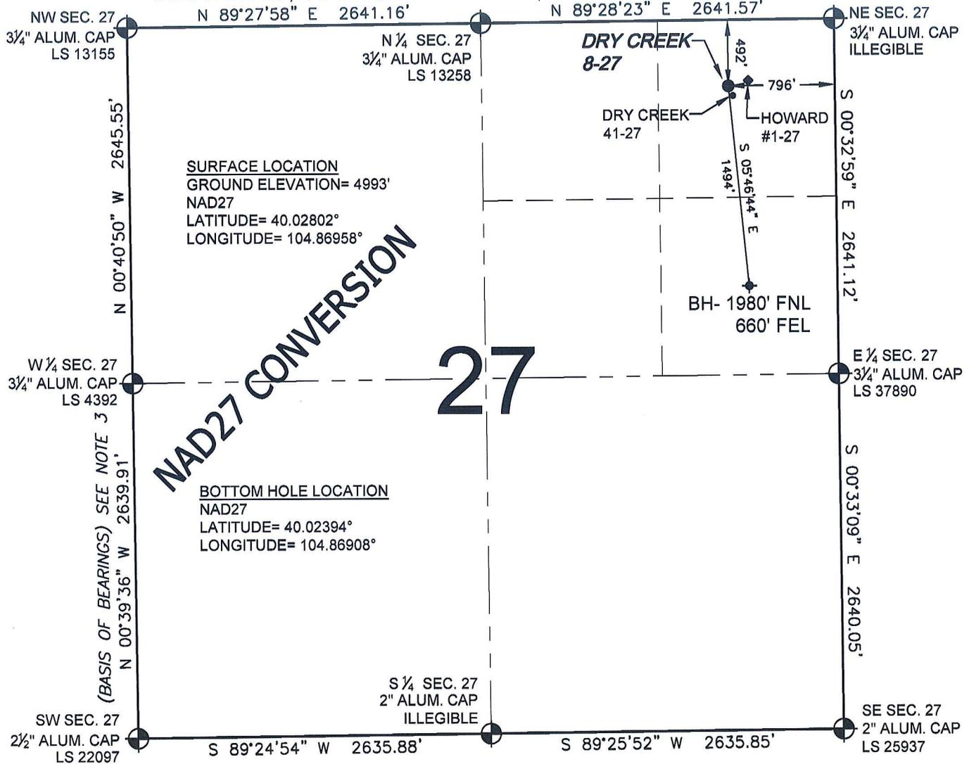
WELL DRY CREEK 8-27 TO BE LOCATED 492' FNL AND 796' FEL, SECTION 27, T1N, R67W OF THE 6th P.M.
