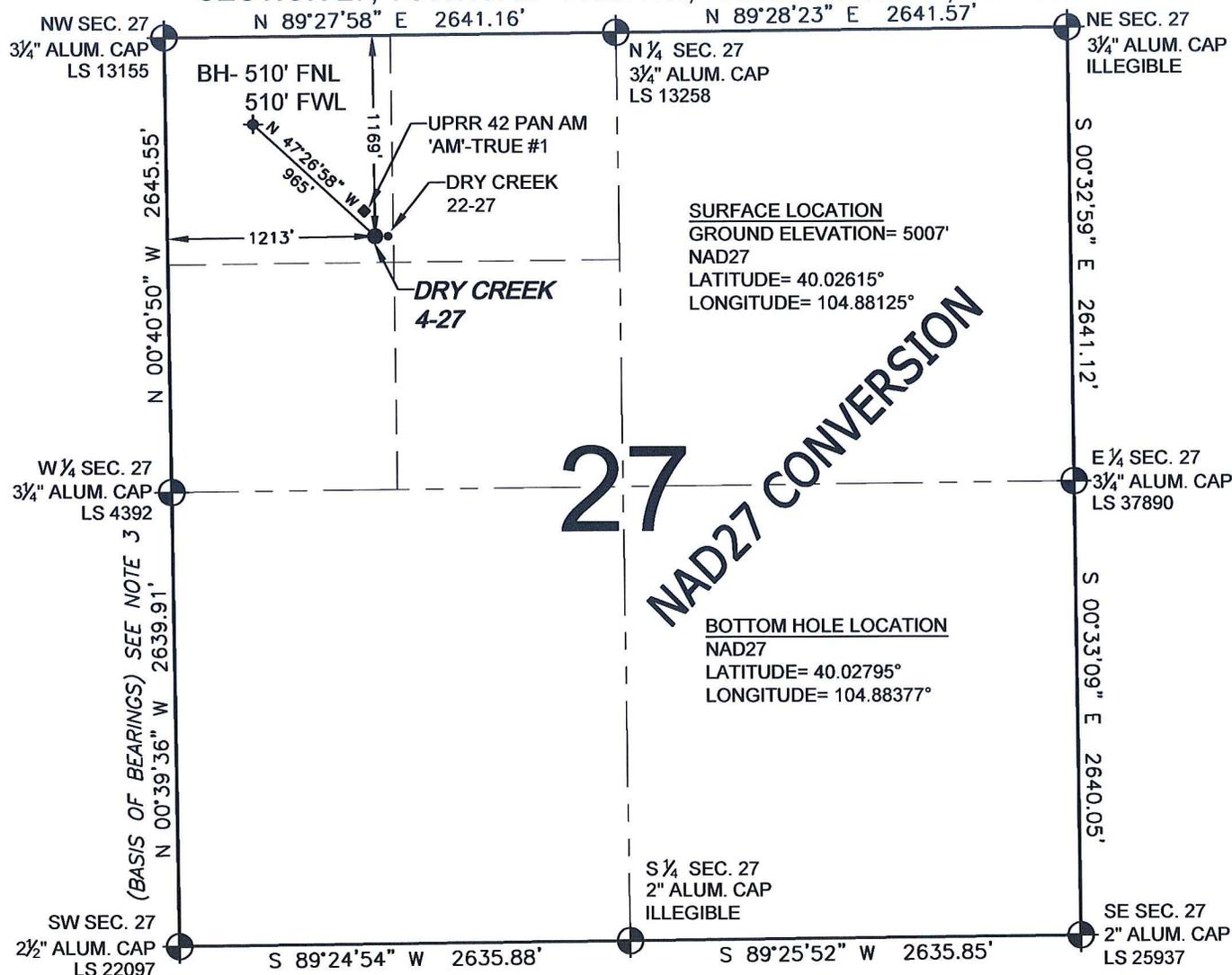
WELL DRY CREEK 4-27 TO BE LOCATED 1169' FNL AND 1213' FWL, SECTION 27, T1N, R67W OF THE 6th P.M.
