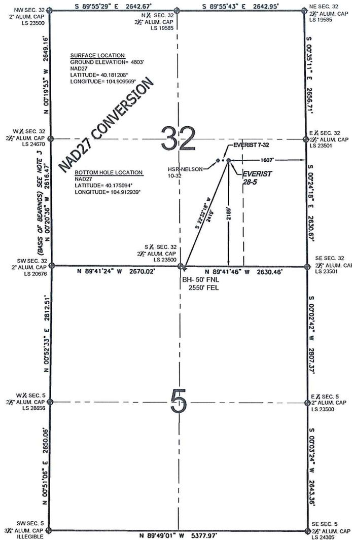
WELL **EVERIST 28-5** TO BE LOCATED 2189' FSL AND 1607' FEL, SECTION 32, T3N, R67W OF THE 6th P.M.
