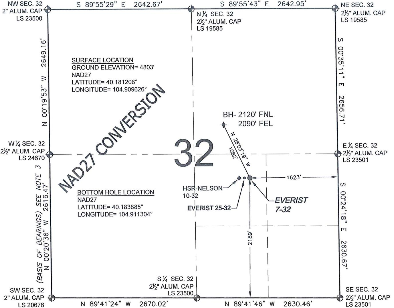
WELL EVERIST 7-32 TO BE LOCATED 2189' FSL AND 1623' FEL, SECTION 32, T3N, R67W OF THE 6th P.M.
