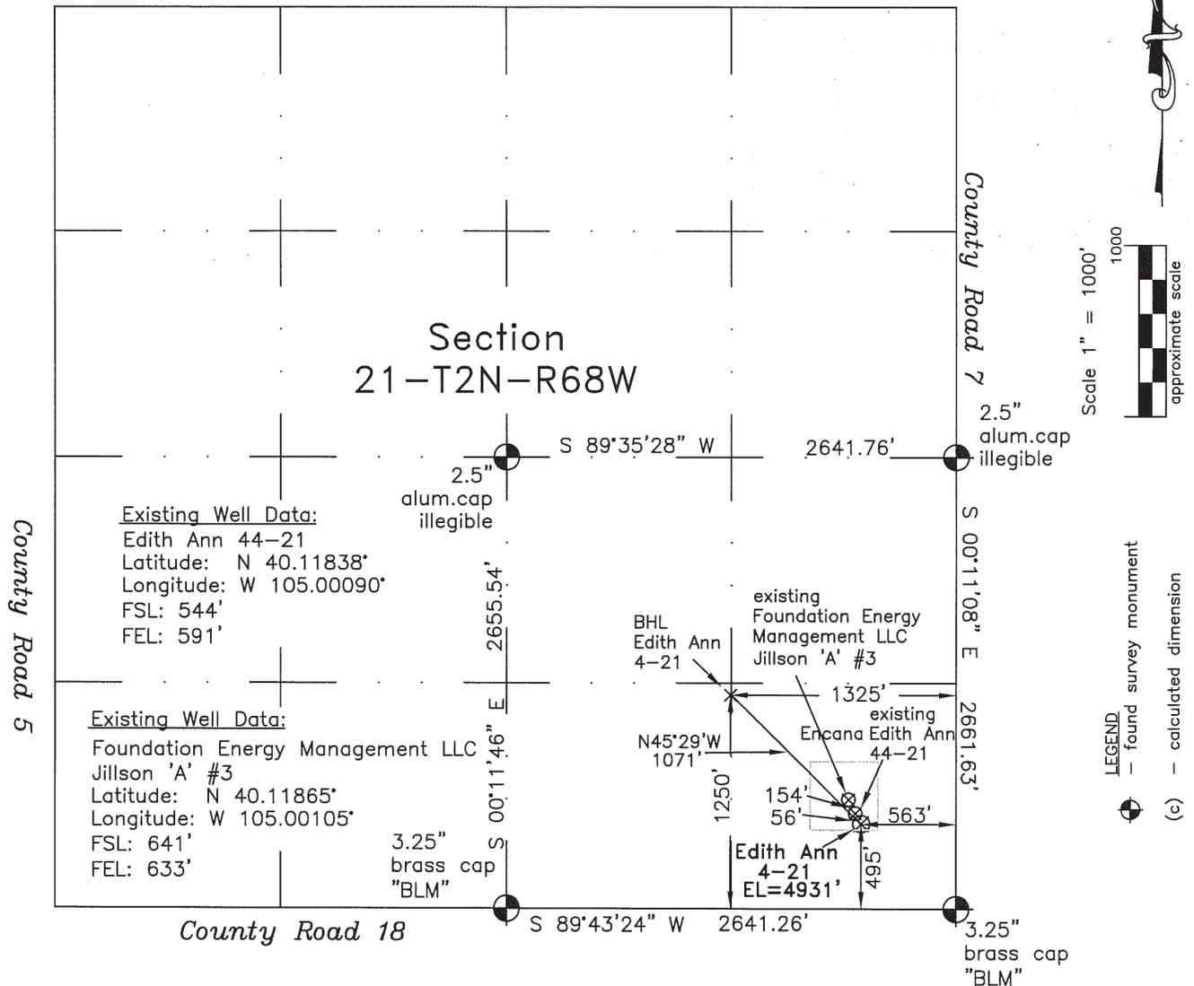
In accordance with a request from Doug Pearlman of EnCana Oil & Gas (USA) Inc., Frederick Land Surveying, Inc. has determined the location of the **Edith Ann 4-21** well site to be SHL: 495' FSL and 563' FEL, (BHL 1250' FSL and 1325' FEL), as measured at ninety (90) degrees from the section lines of Section 21, Township 2 North, Range 68 West of the 6th Principal Meridian, Weld County Colorado.
