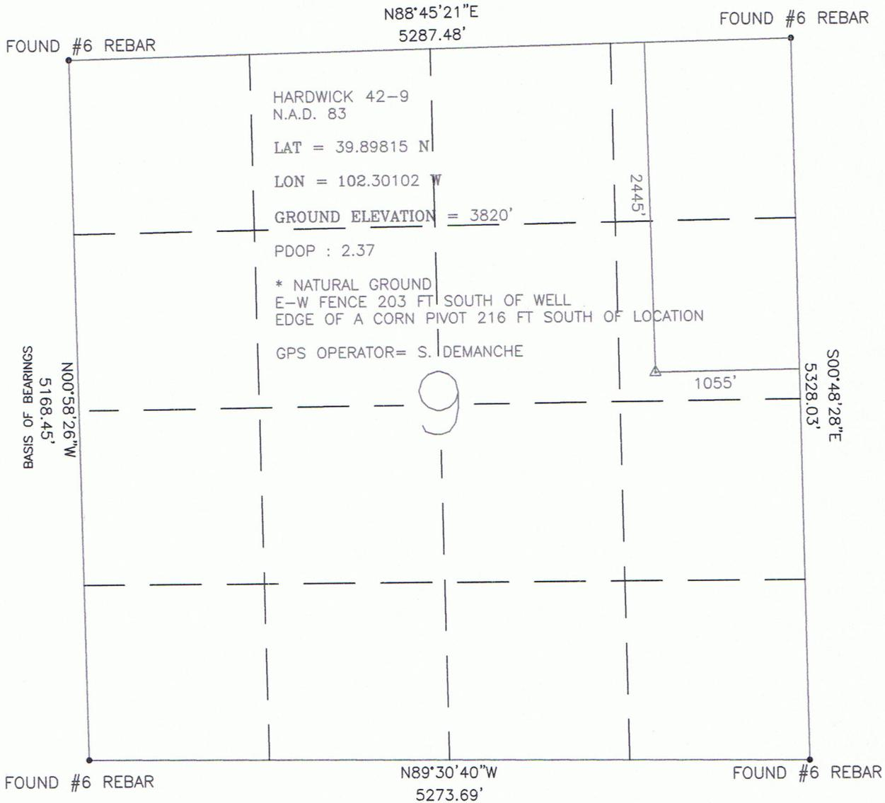
I HEREBY STATETO PETROLEUM DEVELOPMENT CORP THAT THIS WELL LOCATION CERTIFICATE INDICATES THE WELL HARDWICK 42-9 TO BE LOCATED 2445' FNL AND 1055' FEL, SEC 9, T2S, R44W, 6TH P.M. YUMA COUNTY, STATE OF COLORADO
