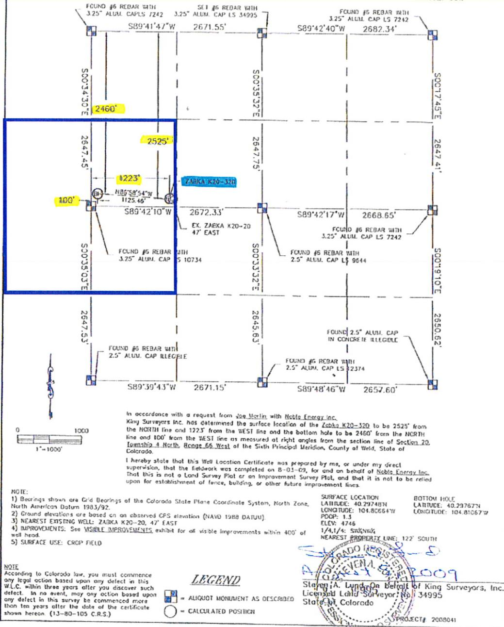
In accordance with a request from Joe Morin with Noble Energy Inc. King Surveyors Inc. has determined the surface location of the Zabka K20-320 to be 2525' from the NORTH line and 1223' from the WEST line and the bottom hole to be 2460' from the NORTH line and 100' from the WEST line as measured at right angles from the section line of Section 20, Township 4 North, Range 66 West of the Sixth Principal Meridian, County of Weld, State of Colorado.
