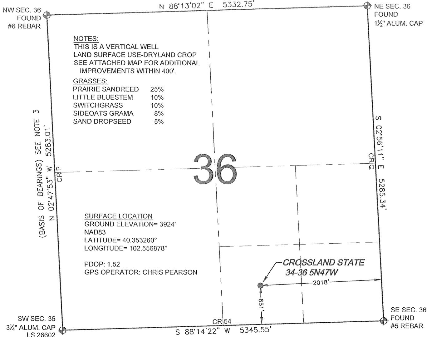
WELL CROSSLAND STATE 34-36 5N47W TO BE LOCATED 651' FSL AND 2018' FEL, SECTION 36, T5N, R47W OF THE 6th P.M.
