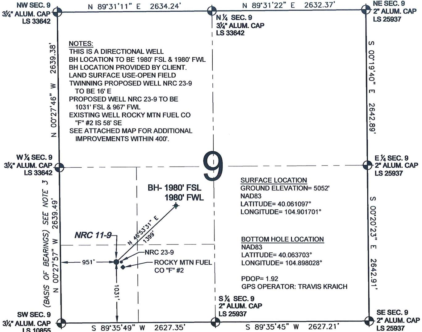
WELL NRC 11-9 TO BE LOCATED 1031' FSL AND 951' FWL, SECTION 9, T1N, R67W OF THE 6th P.M.
