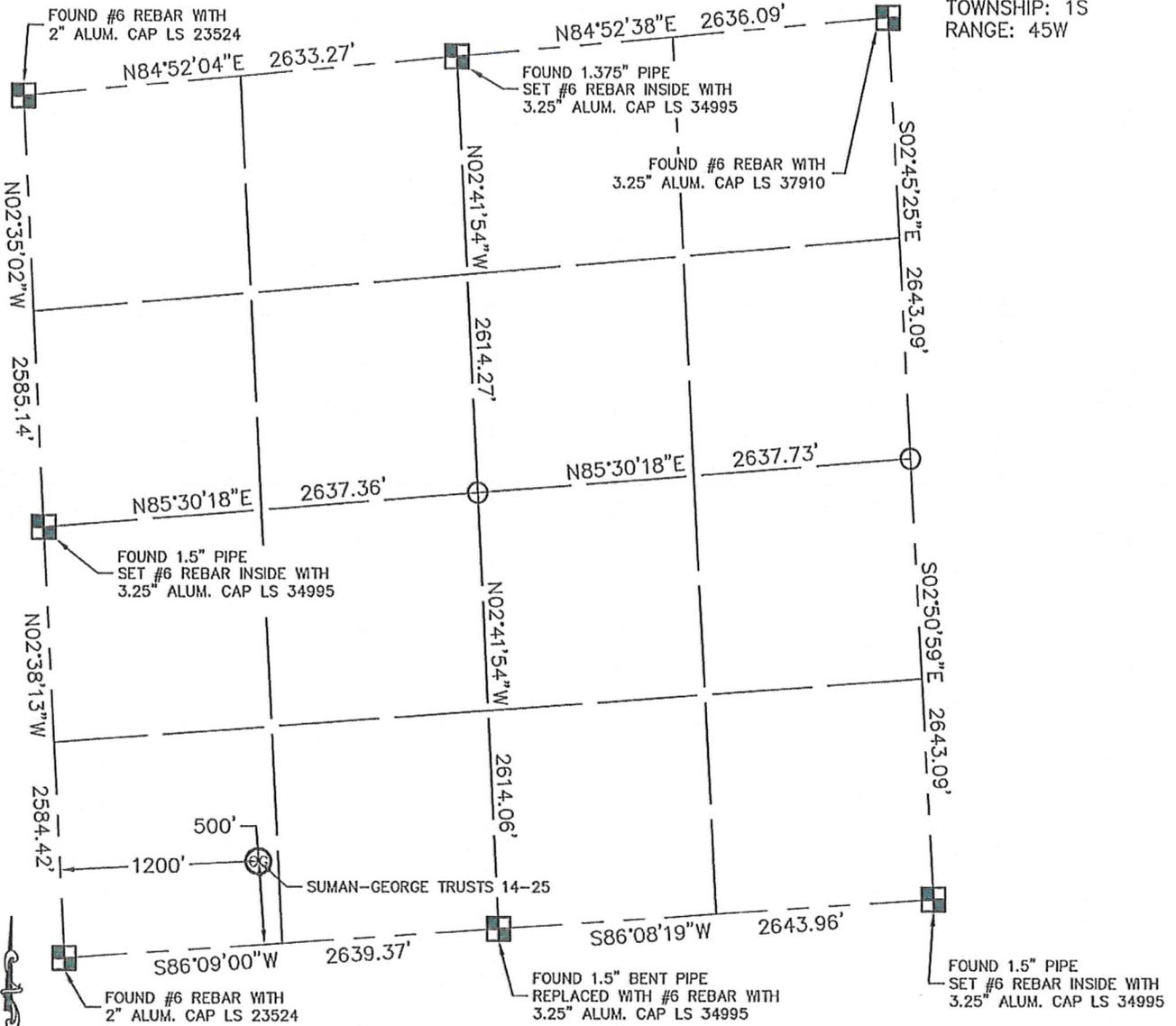
In accordance with a request from Dan Casper with Noble Energy Inc. King Surveyors Inc. has determined the surface location of the SUMAN-GEORGE TRUSTS 14-25 to be 500' from the SOUTH line and 1200' from the WEST line as measured at right angles from the section line of Section 25, Township 1 South, Range 45 West of the Sixth Principal Meridian, County of Yuma, State of Colorado.
