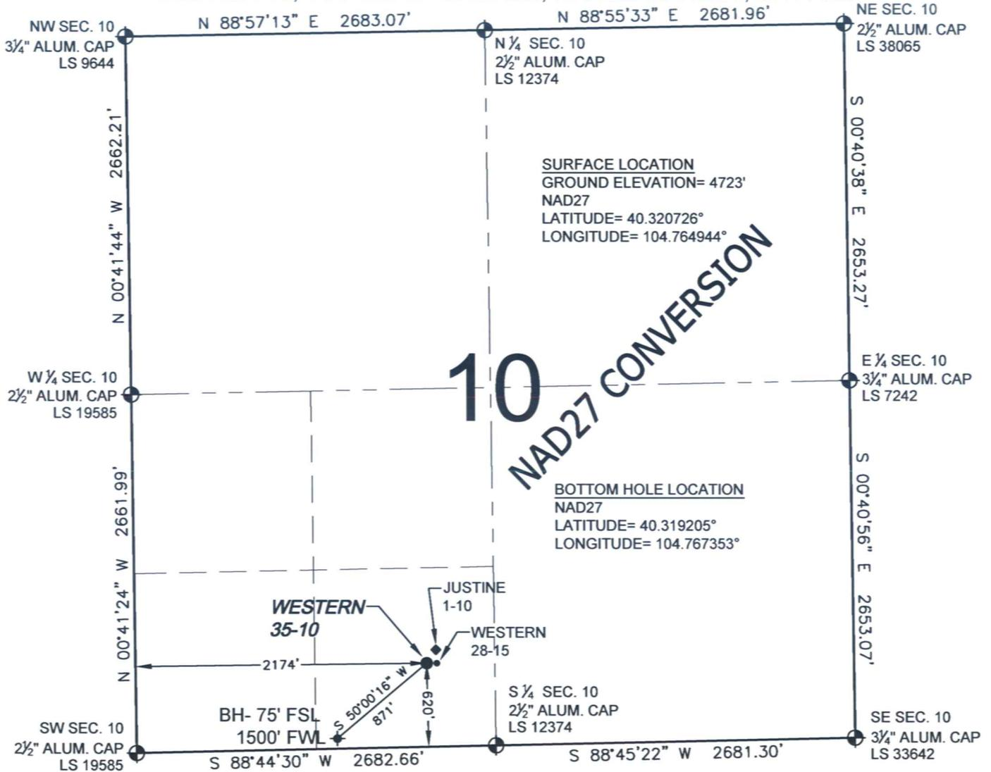
WELL **WESTERN 35-10** TO BE LOCATED 620' FSL AND 2174' FWL, SECTION 10, T4N, R66W OF THE 6th P.M.
