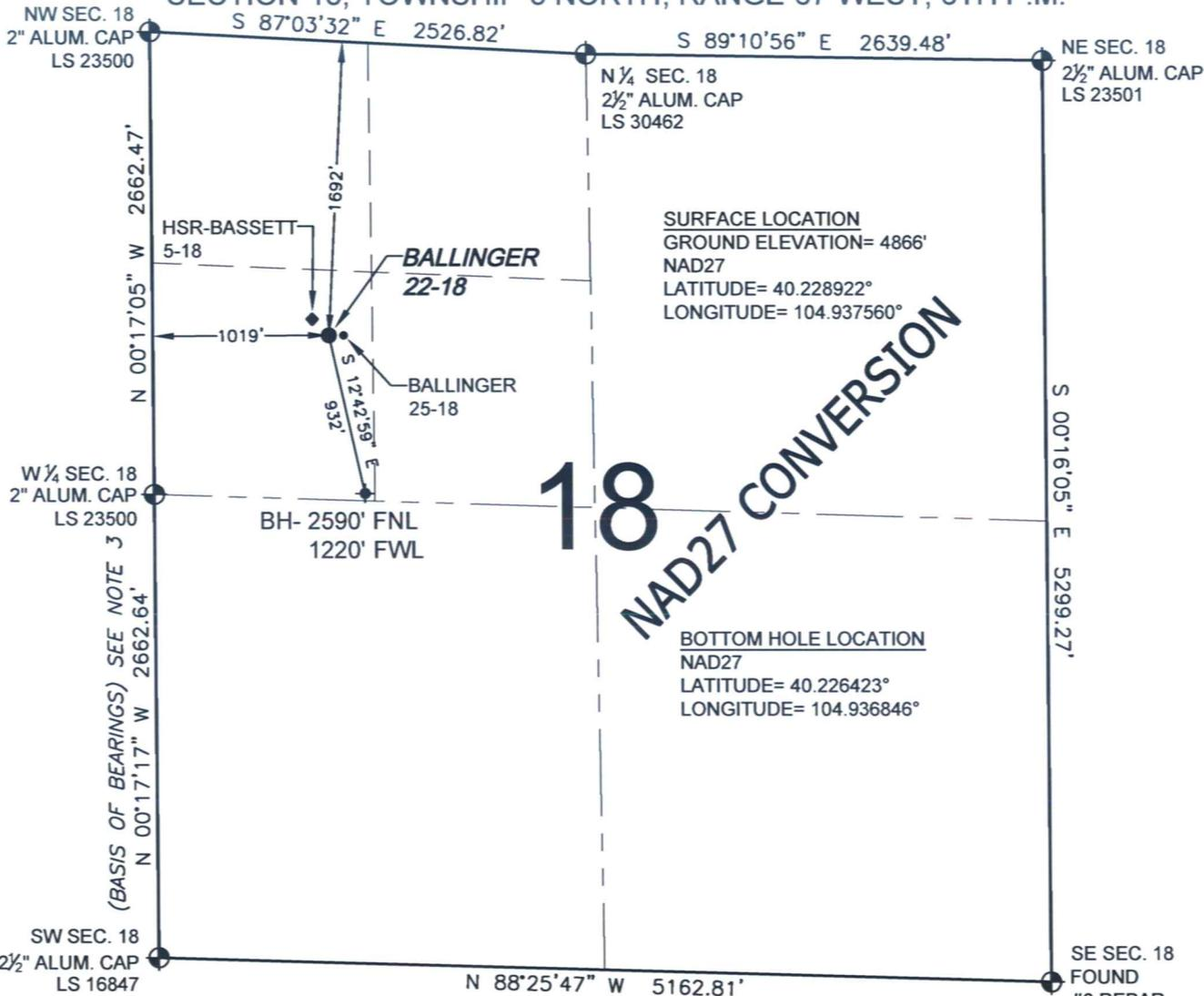
WELL BALLINGER 22-18 TO BE LOCATED 1692' FNL AND 1019' FWL, SECTION 18, T3N, R67W OF THE 6th P.M.
