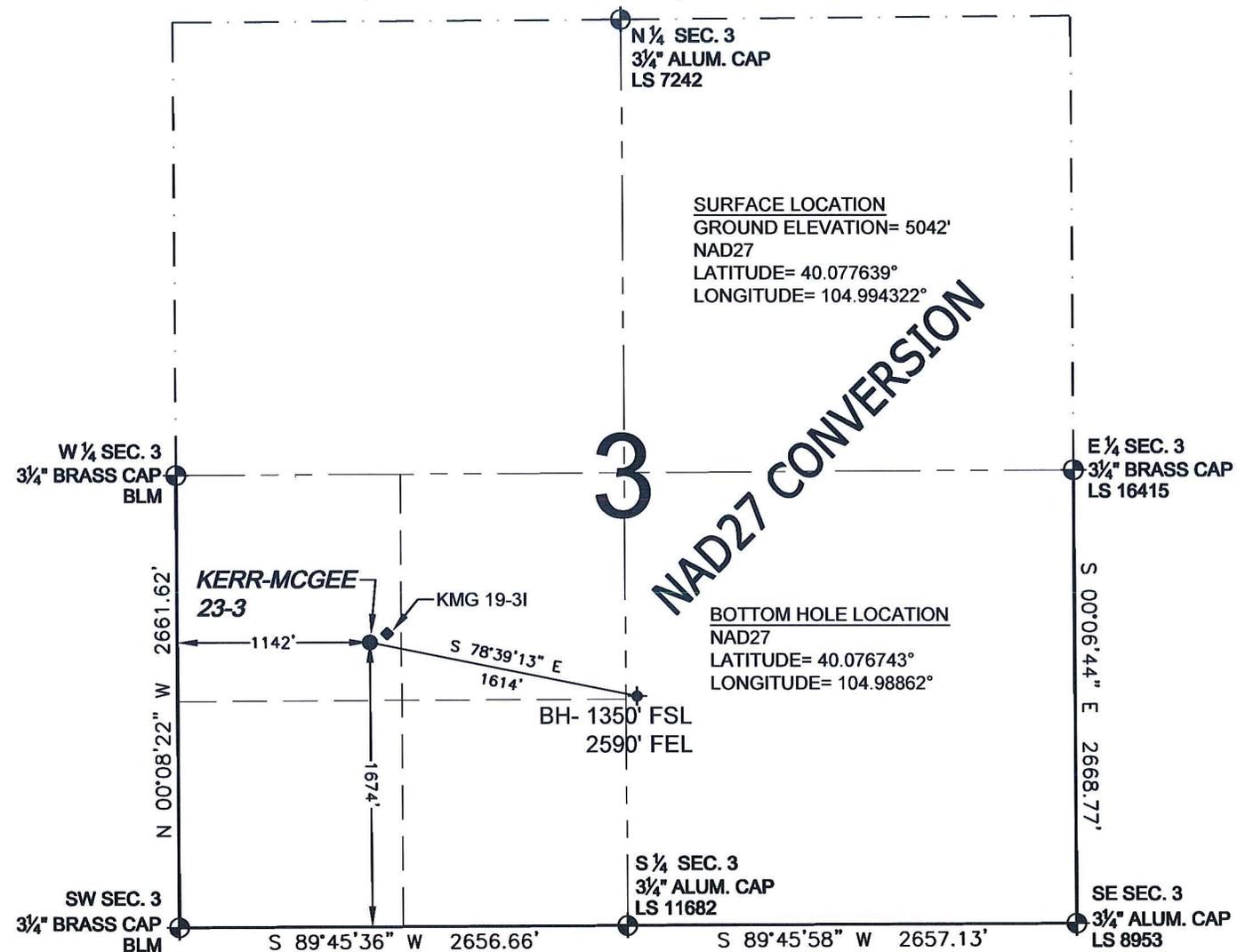
WELL **KERR-MCGEE 23-3** TO BE LOCATED 1674' FSL AND 1142' FWL, SECTION 3, T1N, R68W OF THE 6th P.M.
