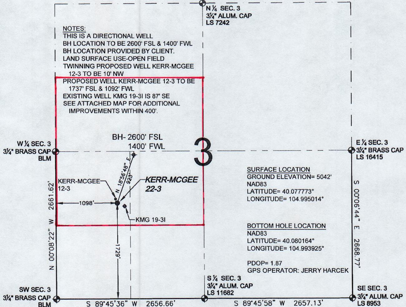
WELL KERR-MCGEE 22-3 TO BE LOCATED 1729' FSL AND 1098' FWL, SECTION 3, T1N, R68W OF THE 6th P.M.
