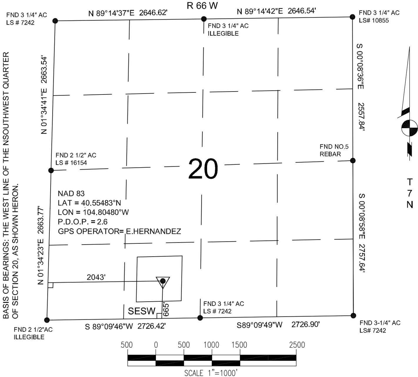
POWER SURVEYING COMPANY, INC. OF FREDERICK, COLORADO HAS IN ACCORDANCE WITH A REQUEST FROM TIM ROBEL OF GREAT WESTERN OIL AND GAS COMPANY DETERMINED THE LOCATION OF LIND 20-24 TO BE 665' FSL & 2043' FWL OF SECTION 20, TOWNSHIP 7 NORTH, RANGE 66 WEST OF THE 6TH PRINCIPAL MERIDIAN, COUNTY OF WELD, STATE OF COLORADO.
