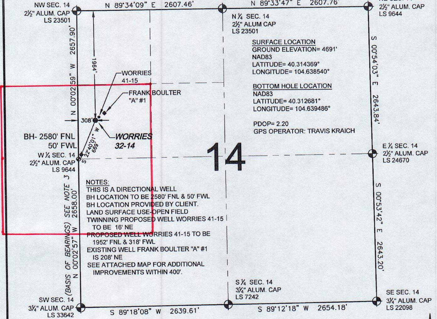
WELL **WORRIES 32-14** TO BE LOCATED 1964' FNL AND 308' FWL, SECTION 14, T4N, R65W OF THE 6th P.M.
