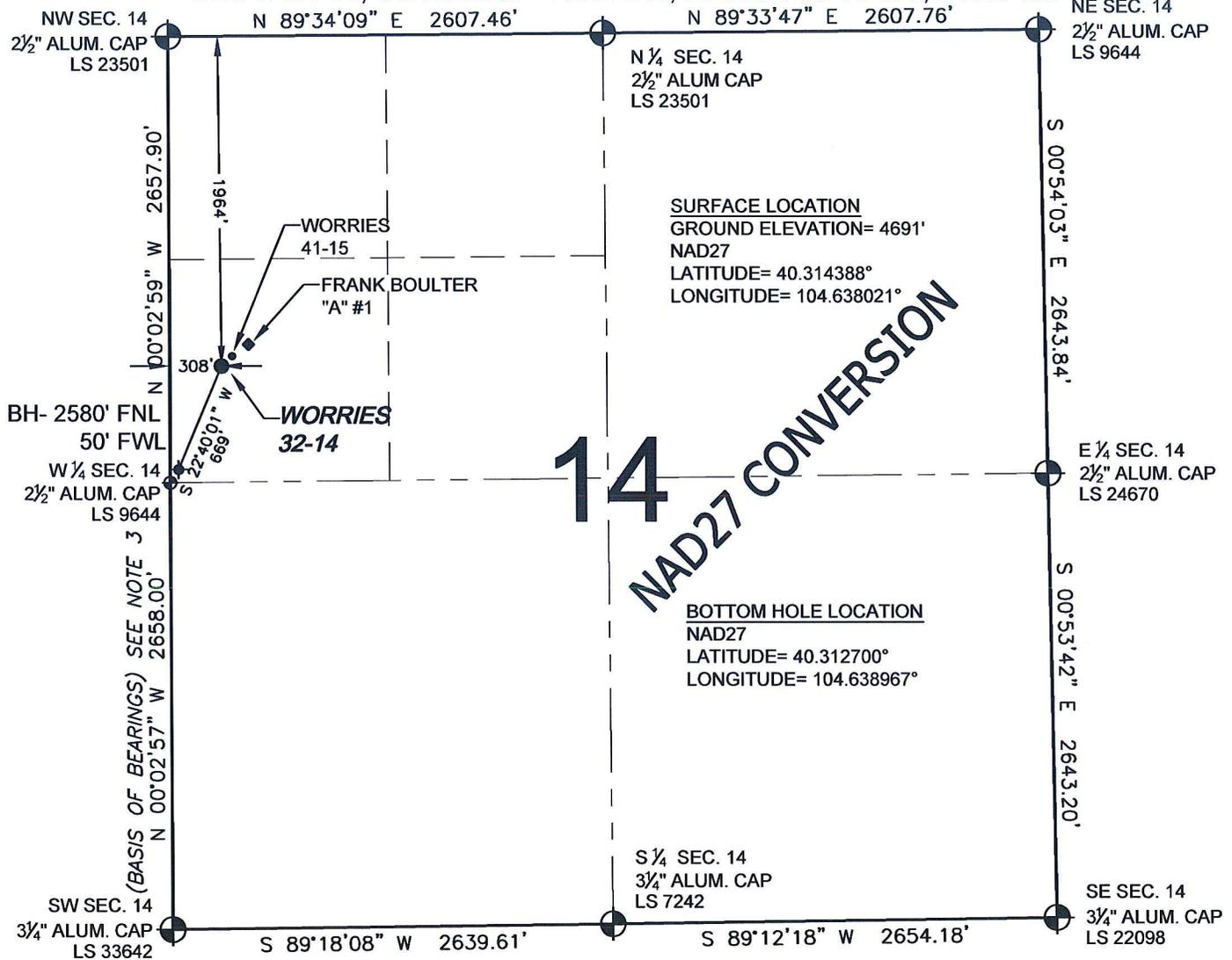
WELL **WORRIES 32-14** TO BE LOCATED 1964' FNL AND 308' FWL, SECTION 14, T4N, R65W OF THE 6th P.M.
