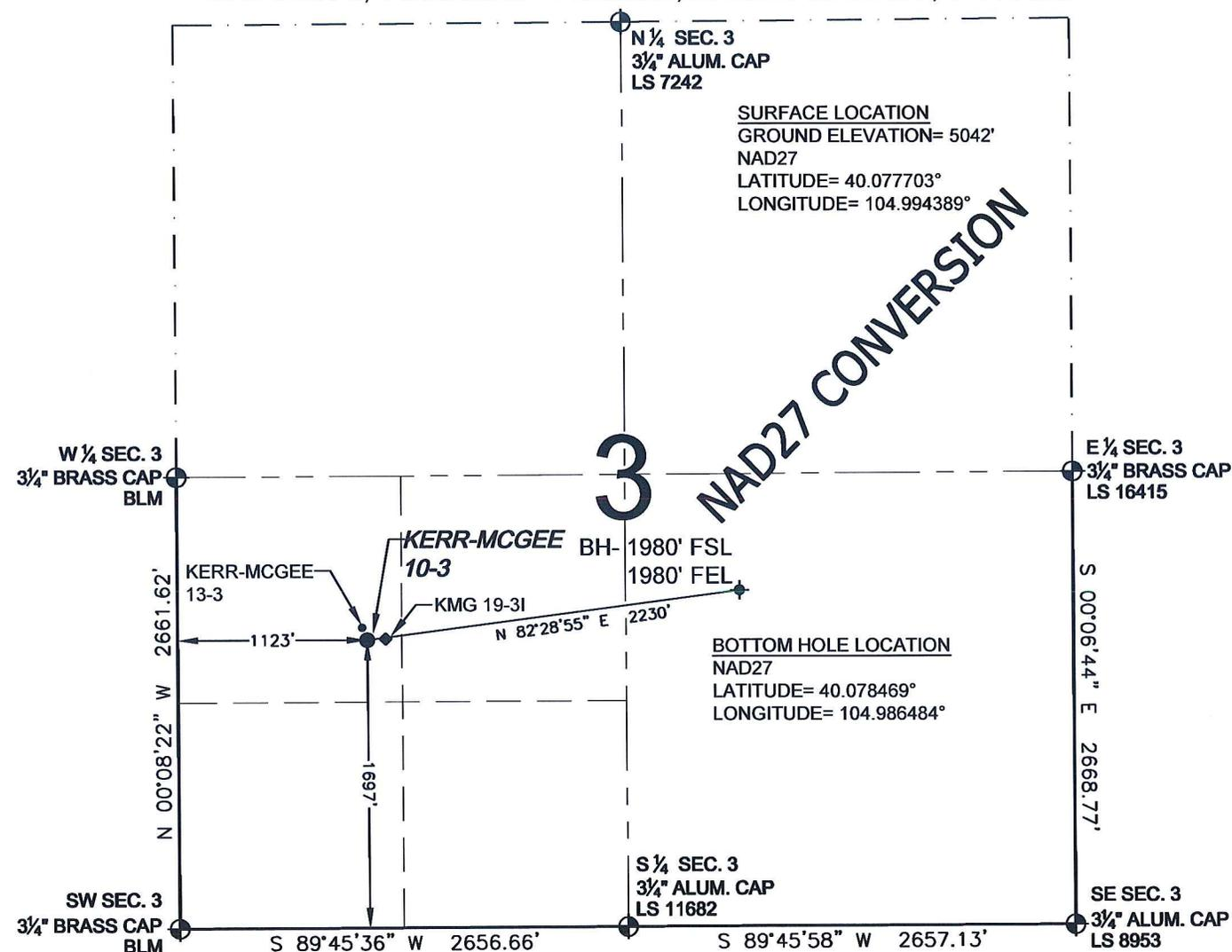
WELL KERR-MCGEE 10-3 TO BE LOCATED 1697' FSL AND 1123' FWL, SECTION 3, T1N, R68W OF THE 6th P.M.
