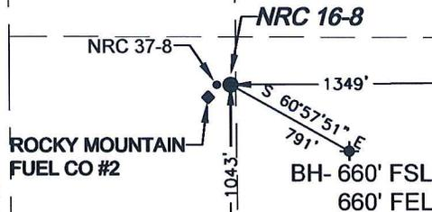
WELL NRC 16-8 TO BE LOCATED 1043' FSL AND 1349' FEL, SECTION 8, T1N, R67W OF THE 6th P.M.
