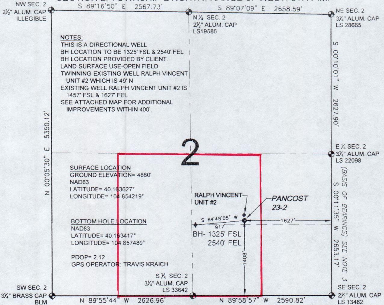
WELL PANCOST 23-2 TO BE LOCATED 1408' FSL AND 1627' FEL, SECTION 2, T2N, R67W OF THE 6TH P.M.
