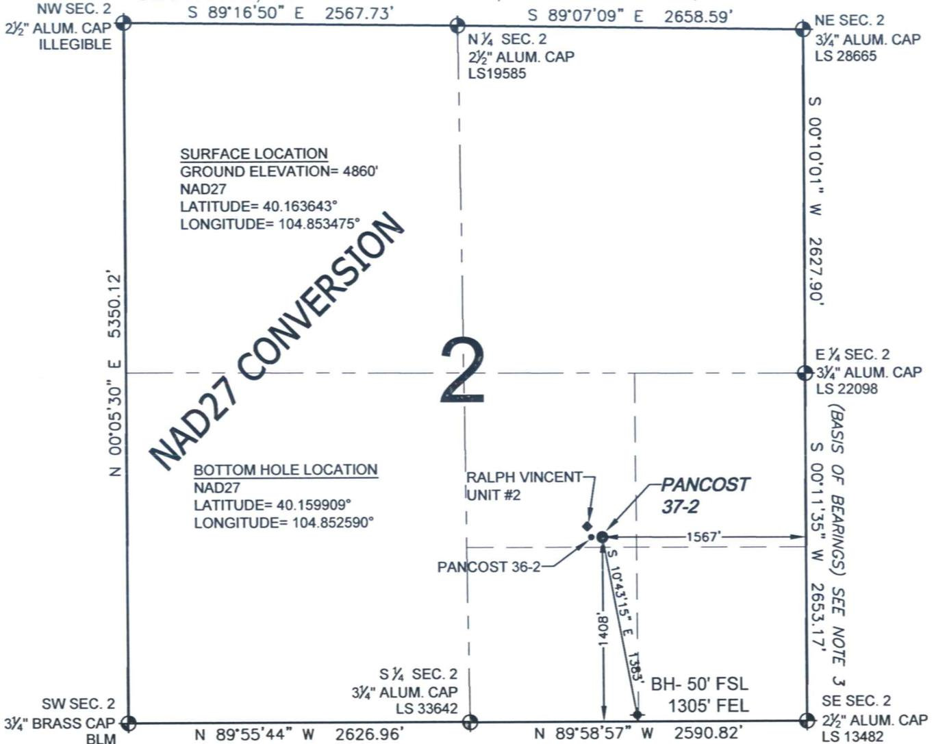
WELL PANCOST 37-2 TO BE LOCATED 1408' FSL AND 1567' FEL, SECTION 2, T2N, R67W OF THE 6th P.M.
