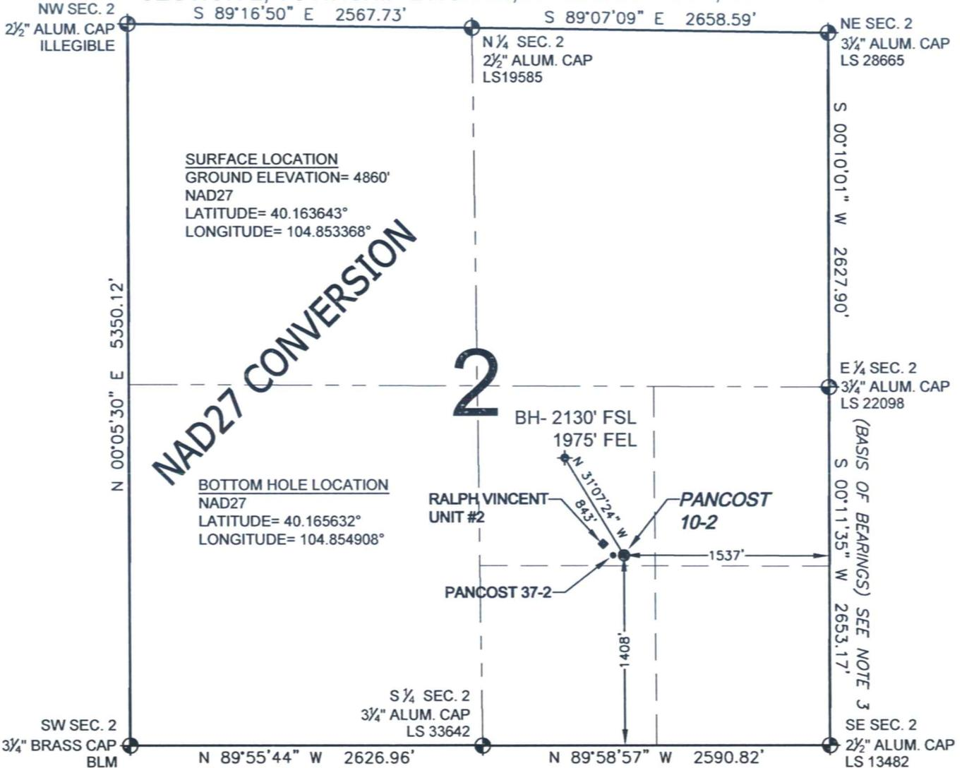
WELL PANCOST 10-2 TO BE LOCATED 1408' FSL AND 1537' FEL, SECTION 2, T2N, R67W OF THE 6th P.M.
