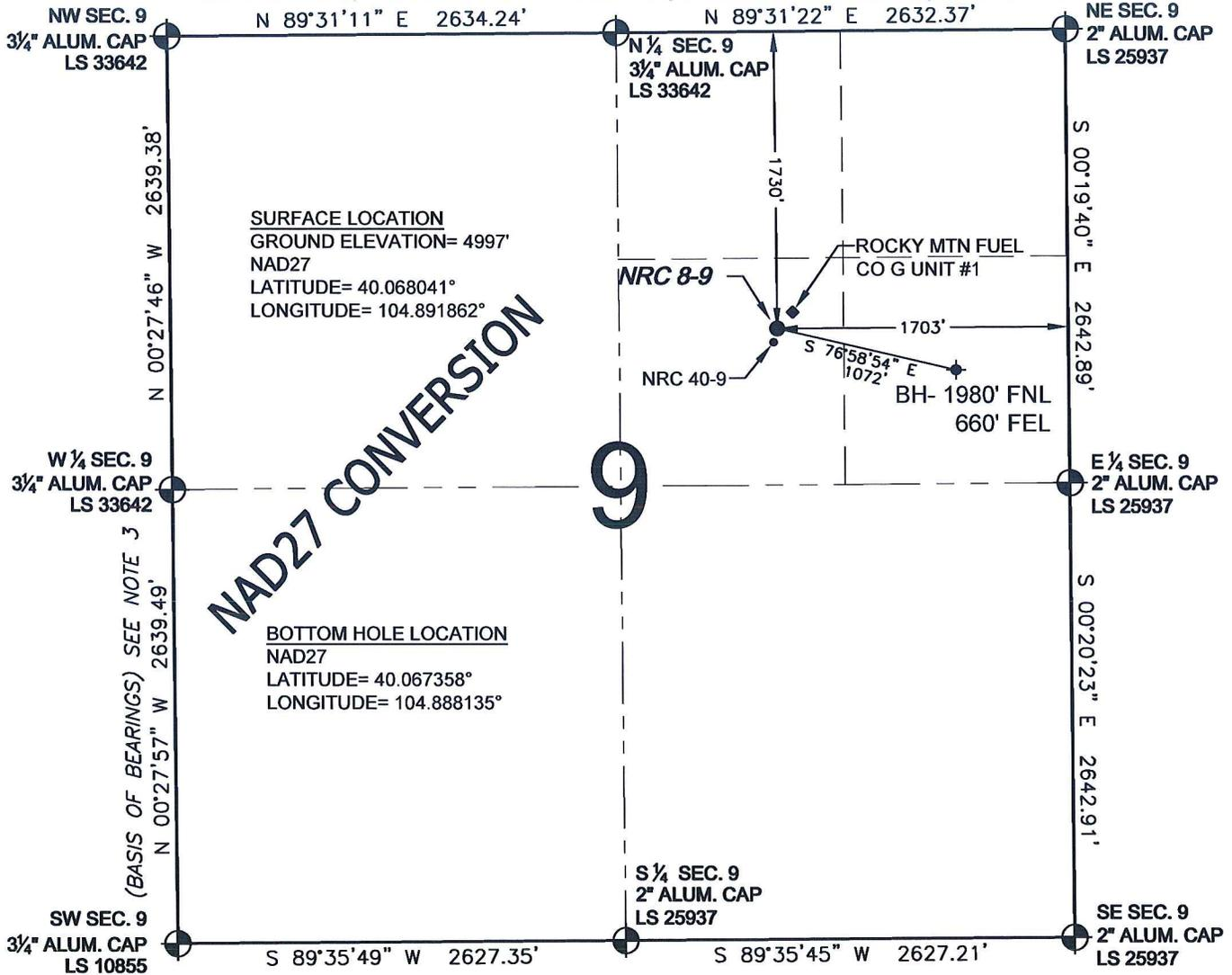
WELL NRC 8-9 TO BE LOCATED 1730' FNL AND 1703' FEL, SECTION 9, T1N, R67W OF THE 6TH P.M.
