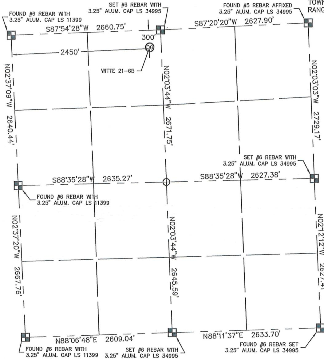
In accordance with a request from Dan Casper with Noble Energy Inc. King Surveyors Inc. has determined the surface location of the WITTE 21-6B to be 300' from the NORTH line and 2450' from the WEST line as measured at right angles from the section line of Section 6, Township 2 South, Range 44 West of the Sixth Principal Meridian, County of Yuma, State of Colorado.
