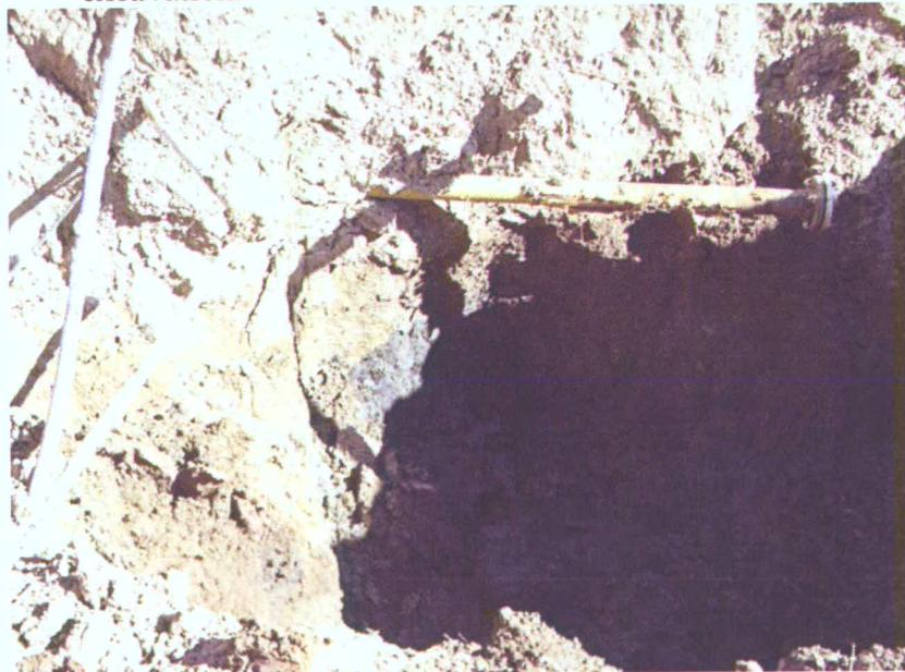
66. Contaminated soils below sump inlet piping.
