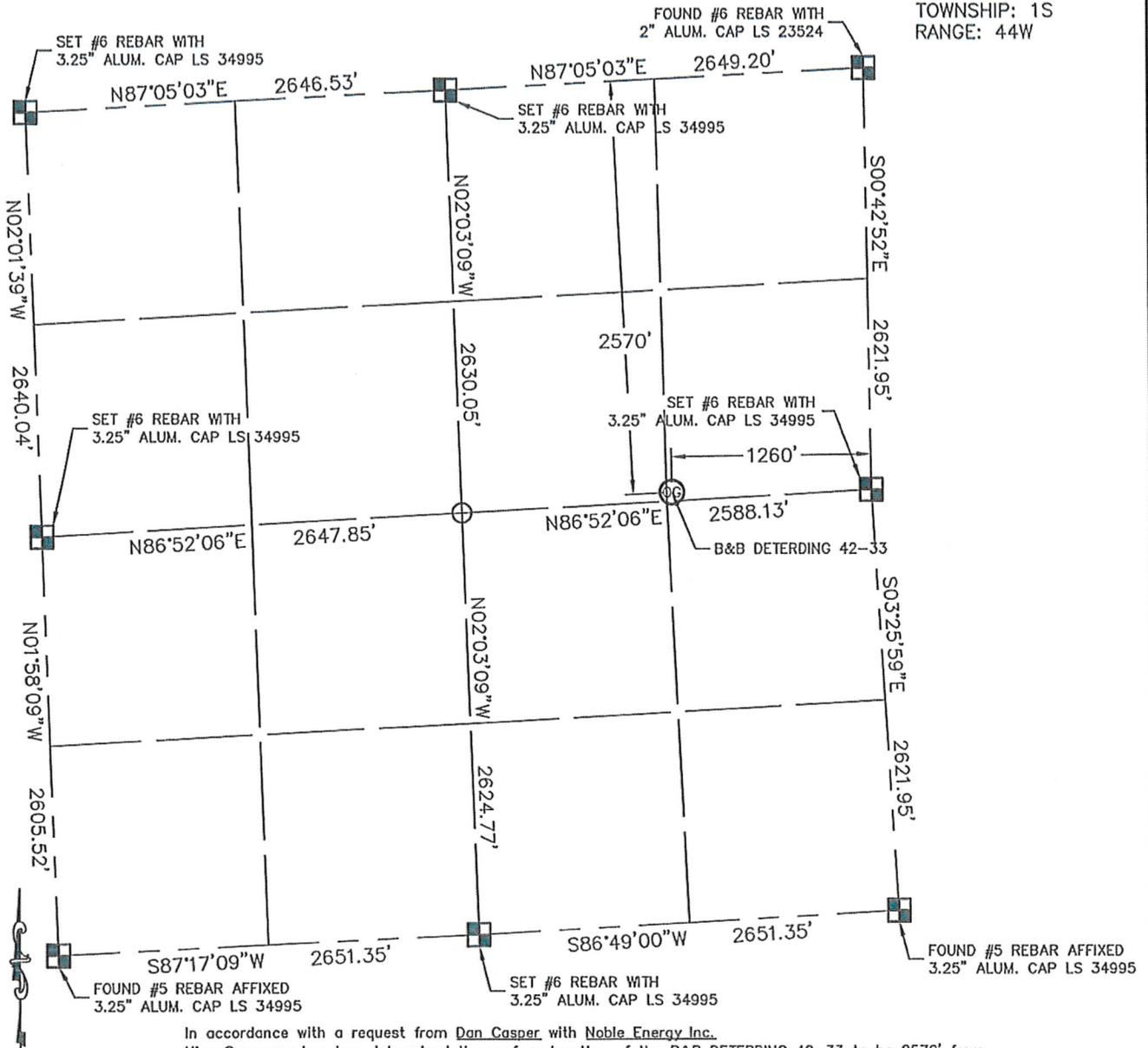
In accordance with a request from Don Casper with Noble Energy Inc. King Surveyors Inc. has determined the surface location of the B&B DETERDING 42-33 to be 2570' from the NORTH line and 1260' from the EAST line as measured at right angles from the section line of Section 33, Township 1 South, Range 44 West of the Sixth Principal Meridian, County of Yuma, State of Colorado.
