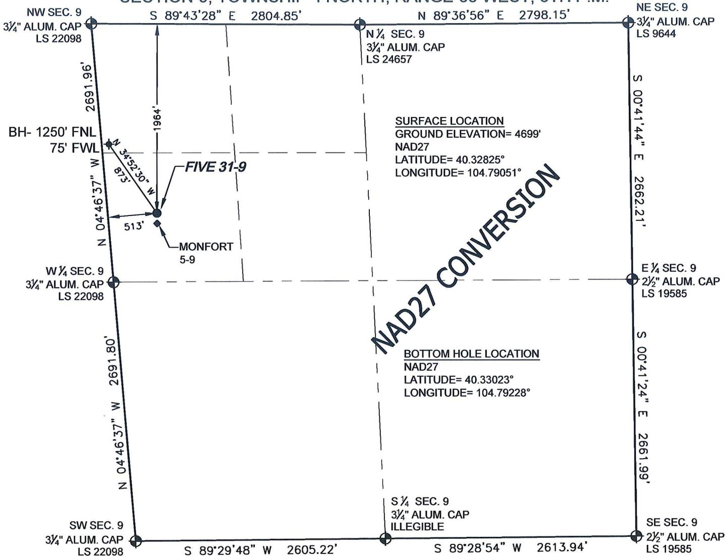
WELL FIVE 31-9 TO BE LOCATED 1964' FNL AND 513' FWL, SECTION 9, T4N, R66W OF THE 6th P.M.
