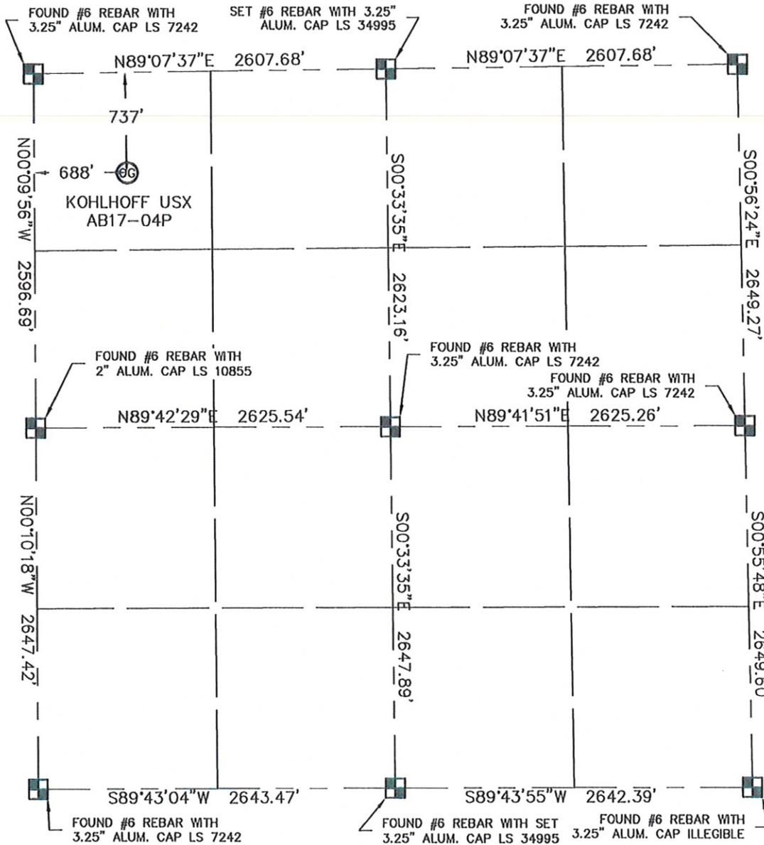
In accordance with a request from Joe Martin with Noble Energy Inc., King Surveyors Inc. has determined the surface location of the Kohlhoff USX AB17-04P to be 737' from the NORTH line and 688' from the WEST line as measured at right angles from the section line of Section 17, Township 7 North, Range 64 West of the Sixth Principal Meridian, County of Weld, State of Colorado.
