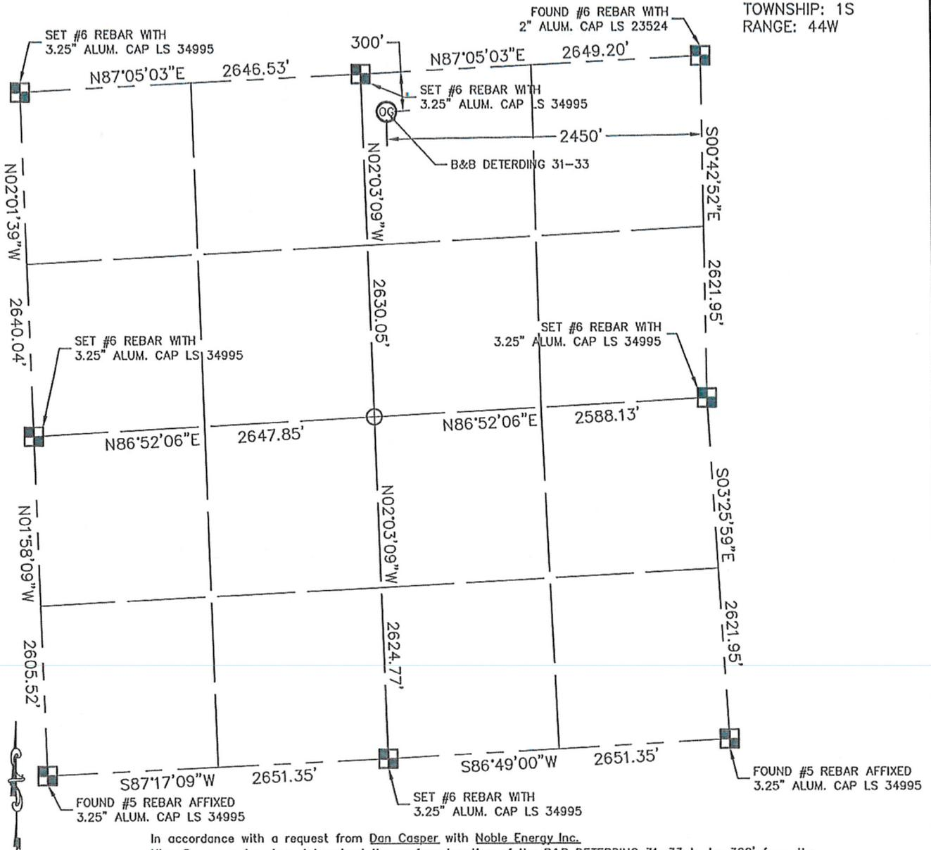
In accordance with a request from Dan Casper with Noble Energy Inc. King Surveyors Inc. has determined the surface location of the B&B DETERDING 31-33 to be 300' from the NORTH line and 2450' from the EAST line as measured at right angles from the section line of Section 33, Township 1 South, Range 44 West of the Sixth Principal Meridian, County of Yuma, State of Colorado.
