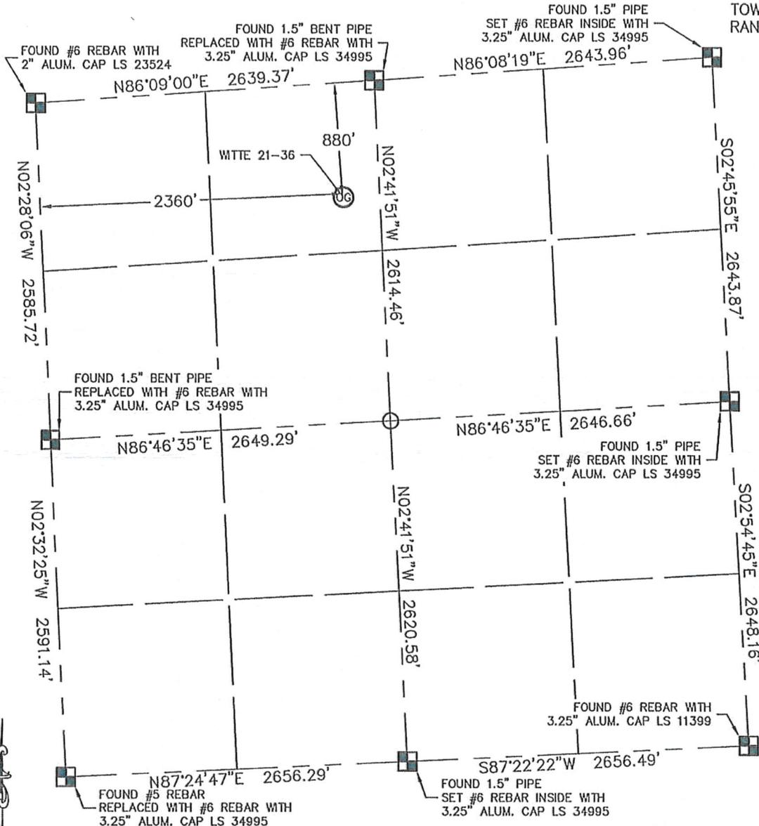
In accordance with a request from Dan Casper with Noble Energy Inc. King Surveyors Inc. has determined the surface location of the WITTE 21-36 to be 880' from the NORTH line and 2360' from the WEST line as measured at right angles from the section line of Section 36, Township 1 South, Range 45 West of the Sixth Principal Meridian, County of Yuma, State of Colorado.
