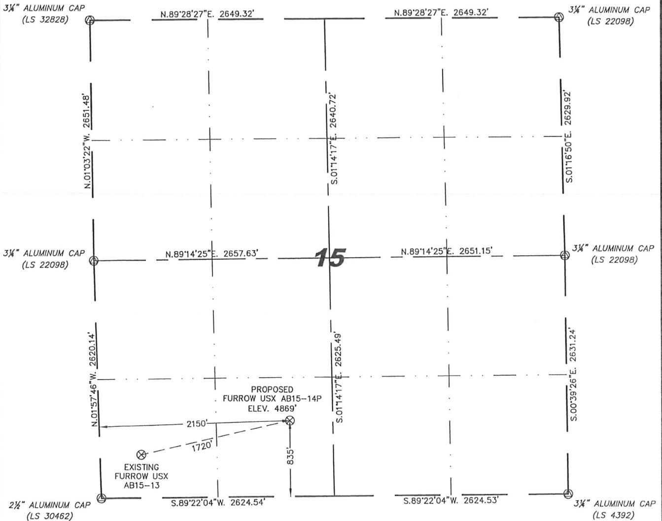
IN ACCORDANCE WITH A REQUEST FROM ERIK VAN DECAR - NOBLE ENERGY INC, STEIL SURVEYING SERVICES, LLC HAS DETERMINED THE LOCATION OF THE FURROW USX AB15-14P WELL TO BE 835' FSL, 2150' FWL, AS MEASURED AT NINETY (90) DEGREES FROM THE SECTION LINES, SECTION 15, TOWNSHIP 7 NORTH, RANGE 64 WEST, 6TH PRINCIPLE MERIDIAN, WELD COUNTY, COLORADO.
