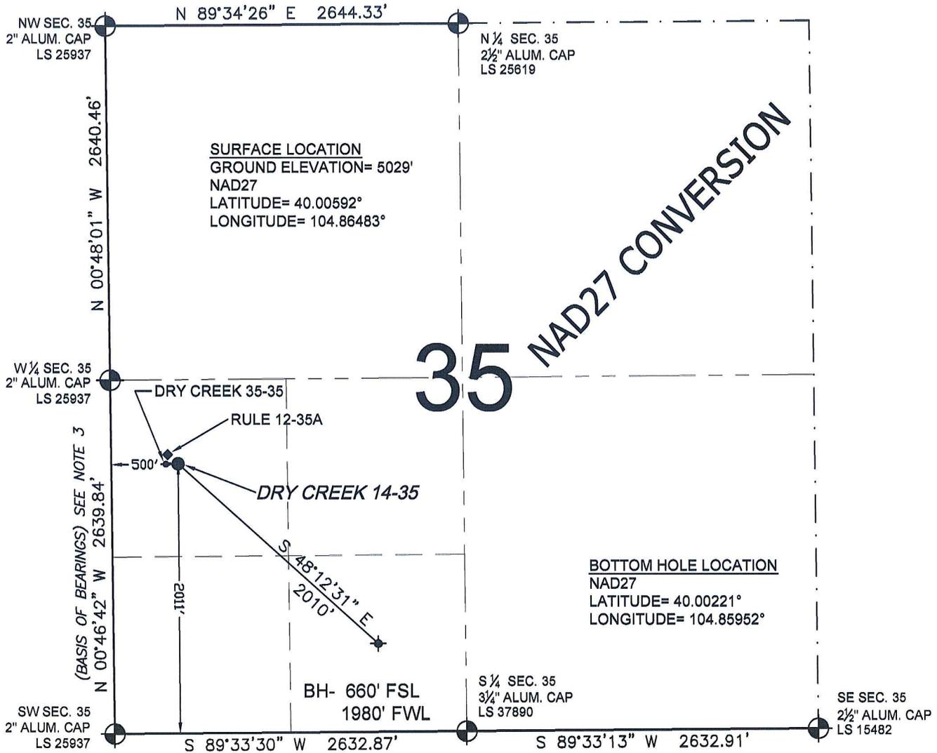
**WELL DRY CREEK 14-35 TO BE LOCATED 2011' FSL AND 500' FWL, SECTION 35, T1N, R67W OF THE 6th P.M.**
